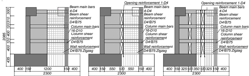
Figure 1. Structural drawing of specimens (W0, W1, and W2 from the left).
