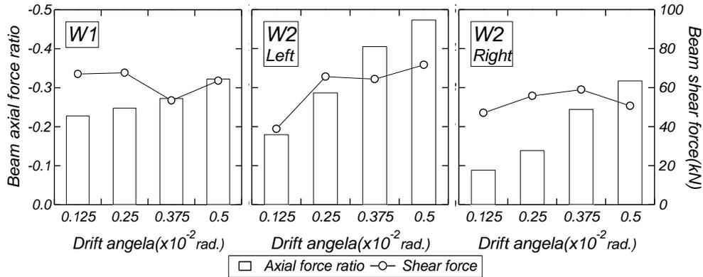
Figure 8. Transitions of total axial and shear forces applied to the boundary beams.
