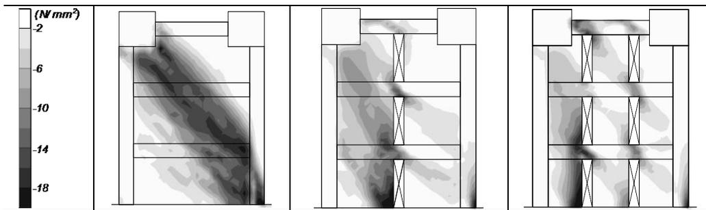
Figure 7. Minimum principle stress contours at 0.5% rad.
