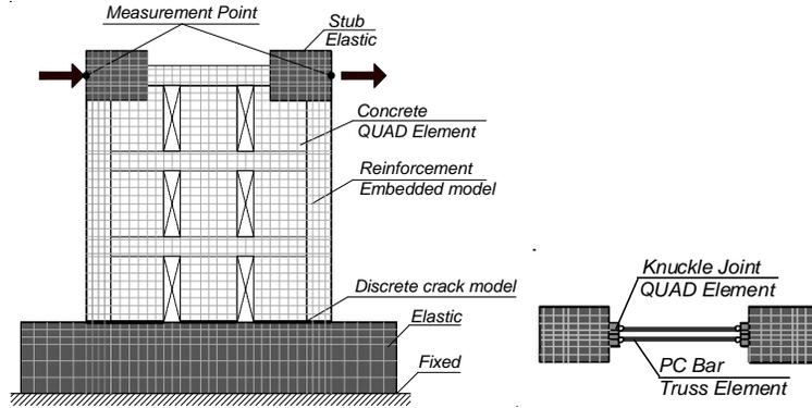
Figure 5. Modeling of W2 for FEM analysis.
