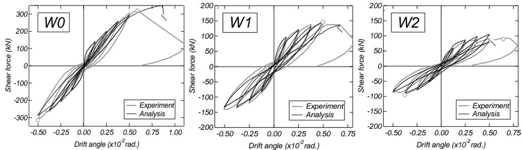
Figure 4. Experimental and analytical shear force-drift angle relationships.
