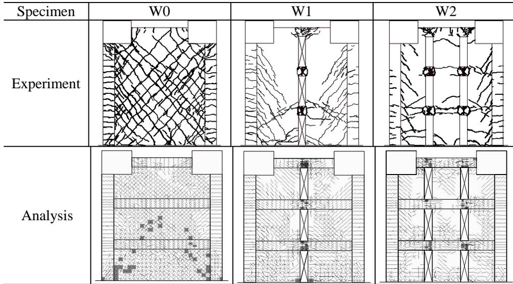
Figure 3. Experimental and analytical damage at 0.5% rad.
