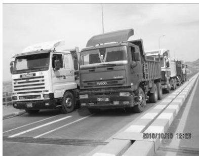
Figure 6. Load test (full load stage).
