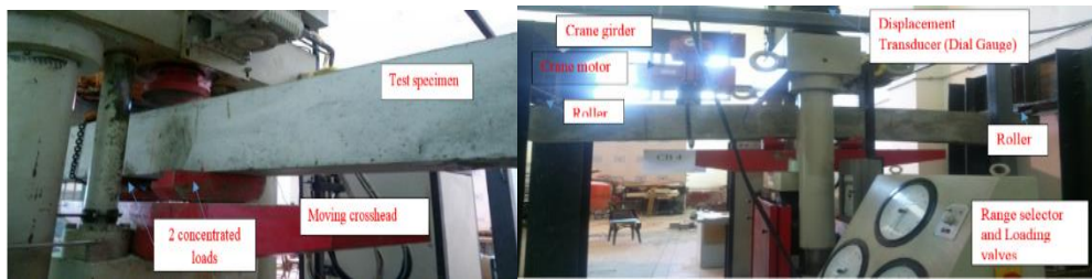
Figure 3. Installation of the samples with the testing machine.
