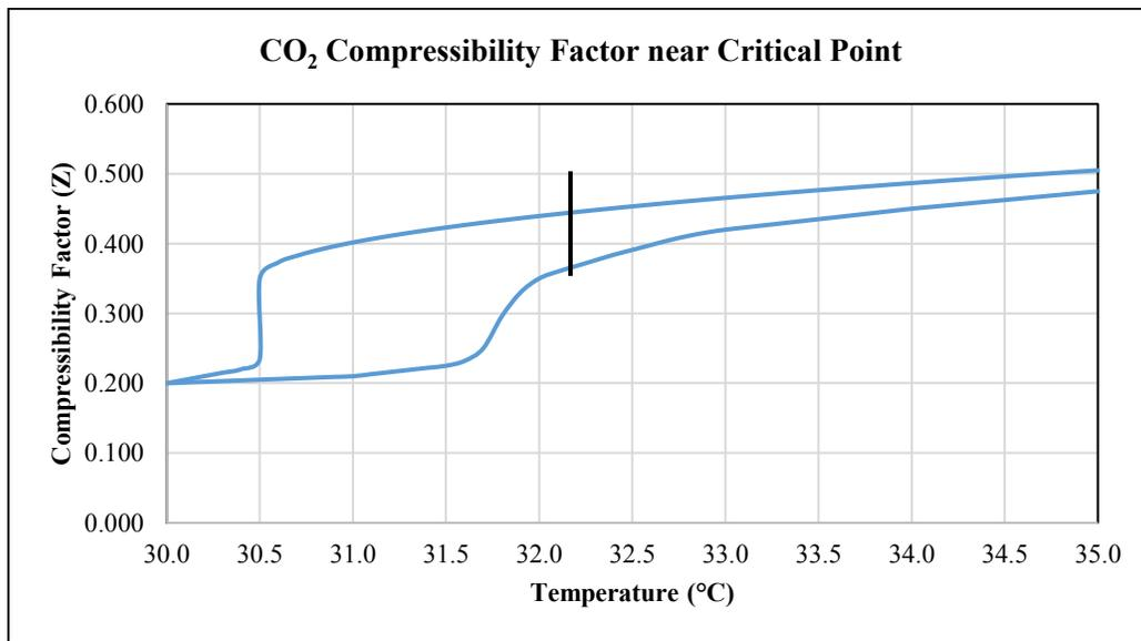
Figure 2. Compressibility factor envelopes for CO<sub>2</sub> near the critical point (Ahn *et al.* 2015).
