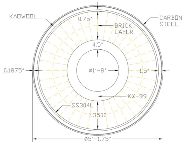
Figure 1. Cross section of the Halotechnics test hot tank (Jonemann 2013).
