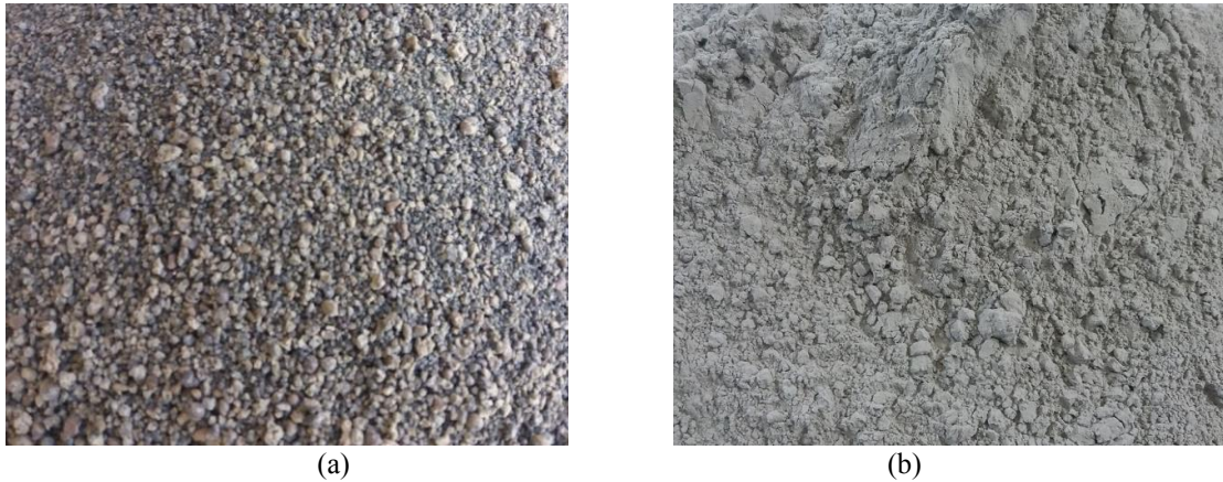
Figure 1. (a) Raw ferronickel slag, (b) Ground ferronickel slag.
