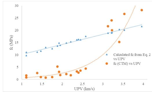
Figure 2. UPV vs. the calculated  $f_c$  and  $f_c$  obtained from the CTM at 28 days.
