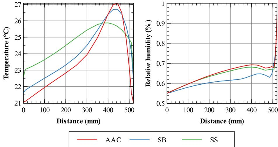
Figure 3. Hygic and moisture profiles as of August 5, 17:00.
