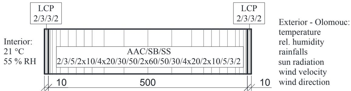
Figure 2. Scheme of analyzed wall.
