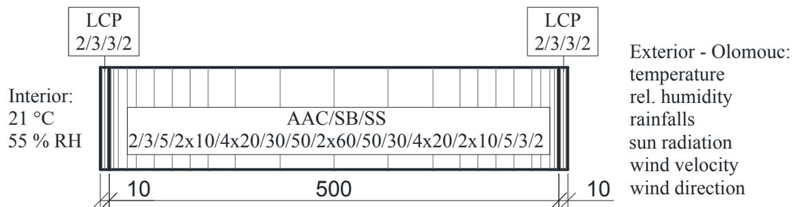
Figure 2. Scheme of analyzed wall.
