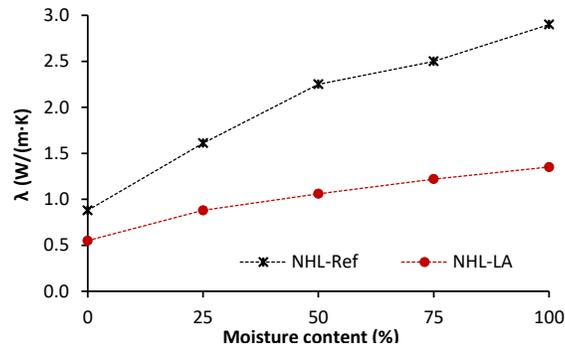
Figure 1. Mortars' moisture dependent thermal conductivity.
