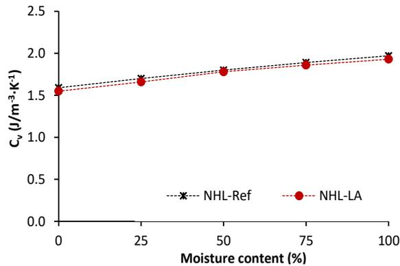
Figure 2. Mortars' moisture dependent heat storage capacity.
