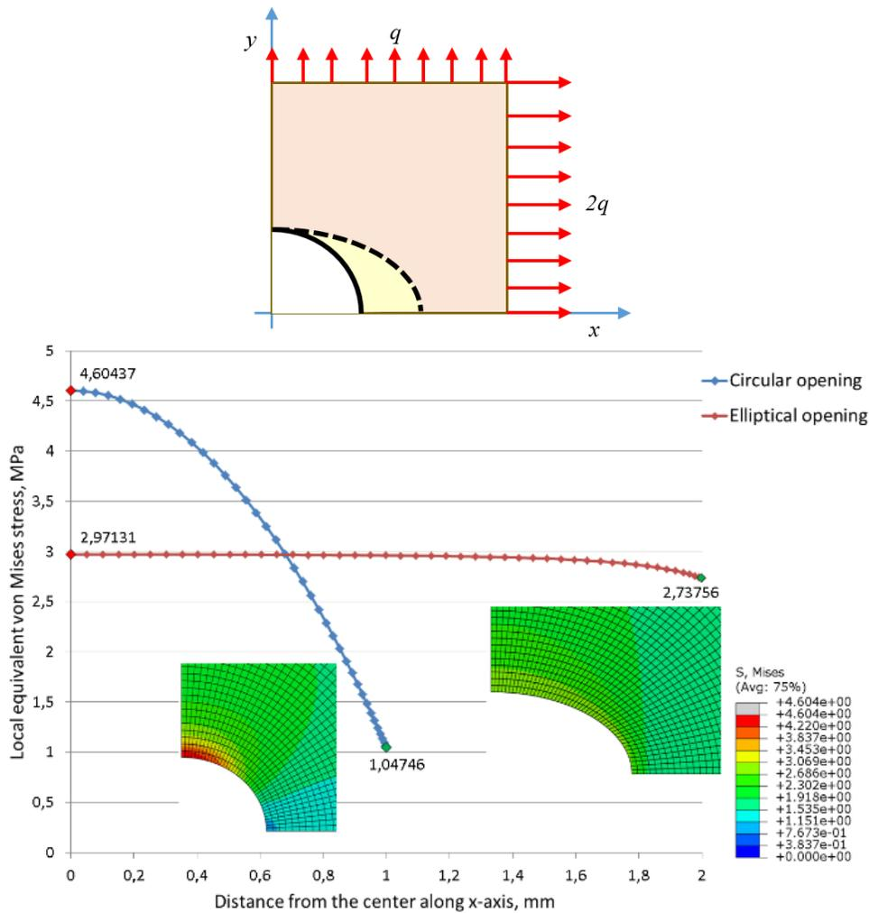
Figure 2. One-quarter of a plate with a central opening (above) and a stress diagram (below) showing the stress levels along the edges of both, the circular and the elliptical opening.
