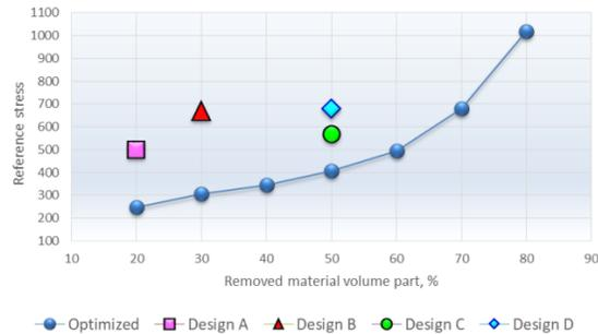
Figure 7. Reference stresses of all optimized designs (curve) and of the 4 recovered design variants (isolated points).
