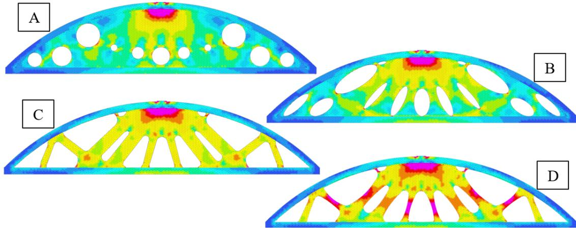
Figure 5. Recovered design variants A, B, C in D; the stress legend ranges from 0 to 500 MPa.
