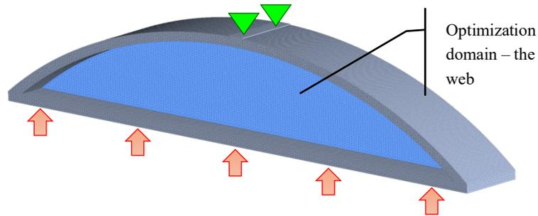
Figure 3. Test bracket; vertically loaded; the web is the optimization domain.
