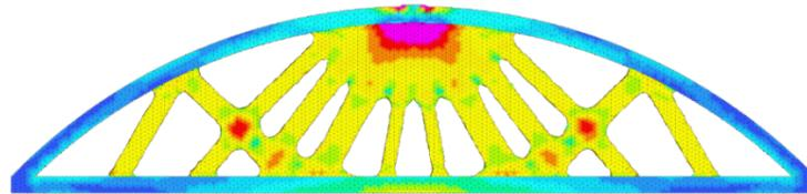
Figure 4. Optimal topology for 50 % volume part of the web; the stress legend ranges from 0 to 500 MPa.
