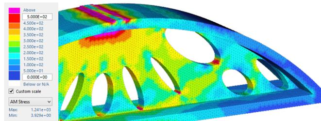
Figure 6. A detail of design B; on cut surfaces one can observe relatively low average stress levels and relatively high-stress concentrations.
