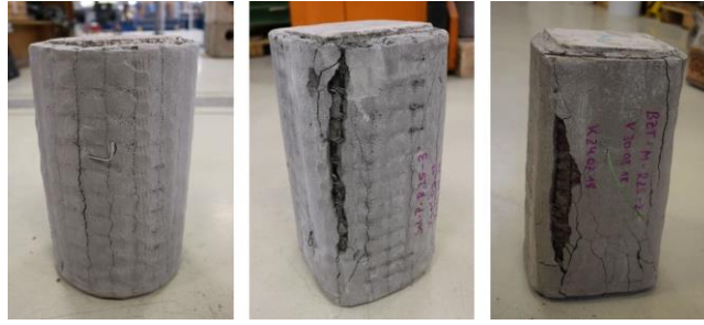
Figure 5. Typical crack pattern of tested specimens.
