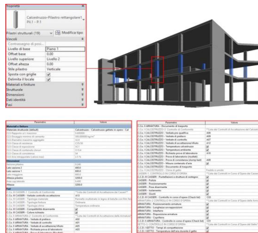
Figure 1. BIM Model (LOD 100) with control sheets.
