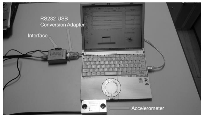
Figure 2. Virtual shaking table test system.
