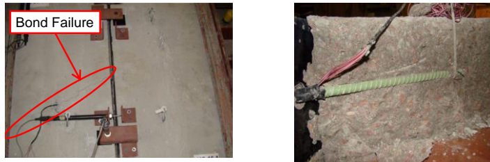
Figure 3. Bond failure in a horizontal skew specimen.
