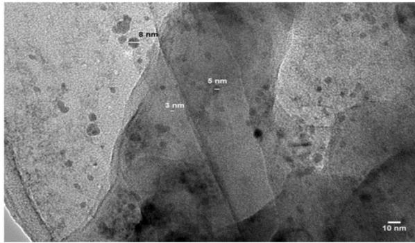
Figure 1. HRTEM images of calcined nanoclay (at 900 °C) at high magnification.
