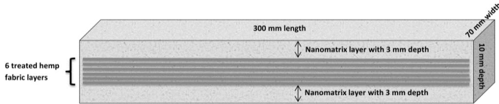
Figure 2. Schematic representation of 6 treated hemp fabric layers position through the depth of cement nanocomposite matrix.
