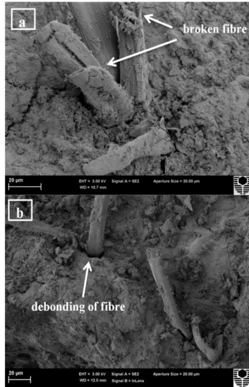
Figure 3. SEM images of the fracture surfaces for: (a) 6THFR-CNCC1, (b) 6THFR-CNCC3 nanocomposites.
