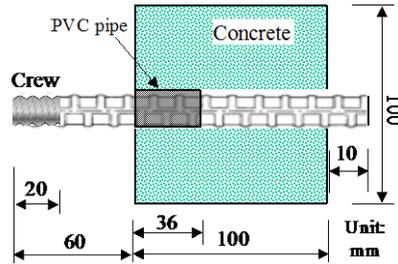
Figure 1. Geometry of the specimen.
