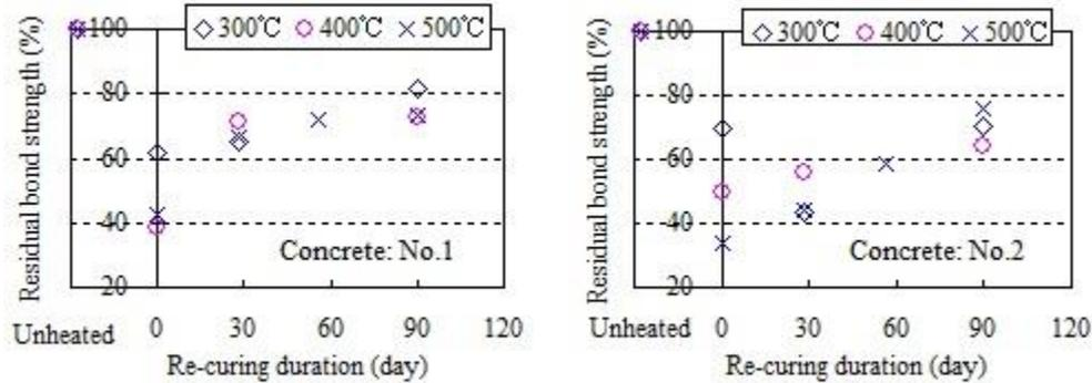
Figure 6. Residual bond strength of concrete exposed to elevated temperature.
