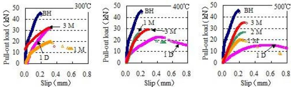
Figure 5. Effects of heating temperature and re-curing duration on the pull-out load – slip relational curve (Series of concrete: No.2).
