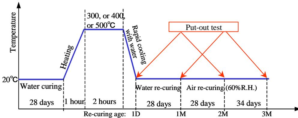
Figure 2. Regime of heating, curing and pull-out test.
