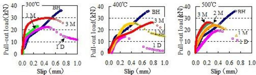
Figure 4. Effects of heating temperature and re-curing duration on the pull-out load – slip relational curve (Series of concrete: No.1).
