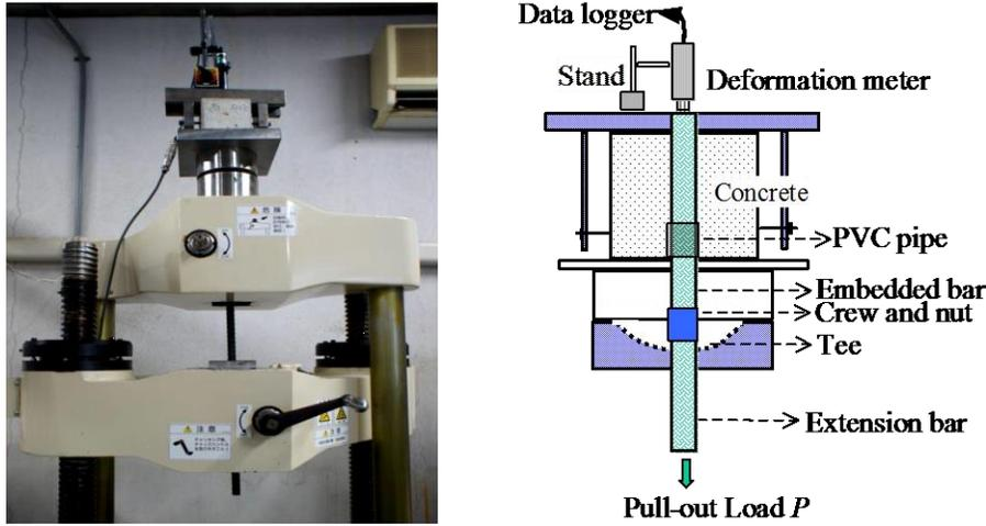
Figure 3. Pull-out test for bond strength measurement.
