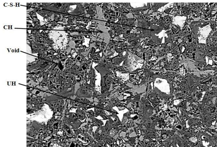
Figure 2. SEM Microstructure of Cement Paste at 28 Days of Curing.
