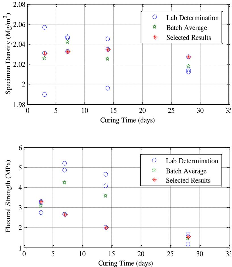
Figure 1. Flexural Test Results for a w/c Ratio of 0.35.
