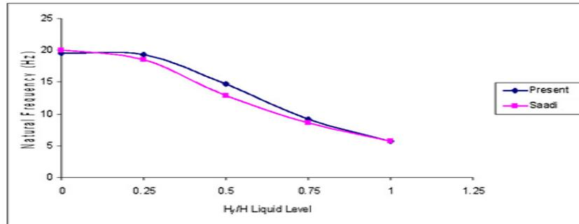
Figure 3. Coupled natural frequency for various filling ratios for tall tank.
