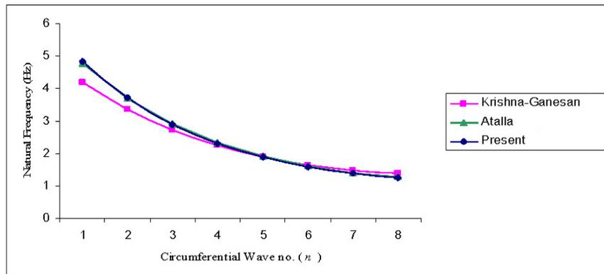
Figure 2. Values of natural frequency compared with previous works.
