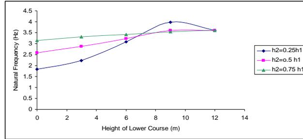
Figure 4. Relation between the natural frequency and height of lower course.
