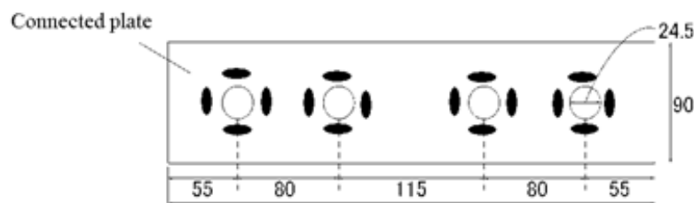
Figure 2. Example of measurement position (splice plate) [unit: mm].
