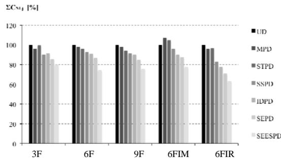
Figure 2. Comparison of the total sum of damping coefficients ( $\xi_{ve1}=20\%$ ).
