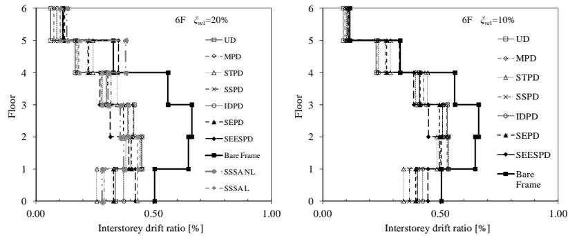
Figure 3. Interstory drifts for frames 6F ( $\xi_{ve1}=20\%$  left;  $\xi_{ve1}=10\%$  right).
