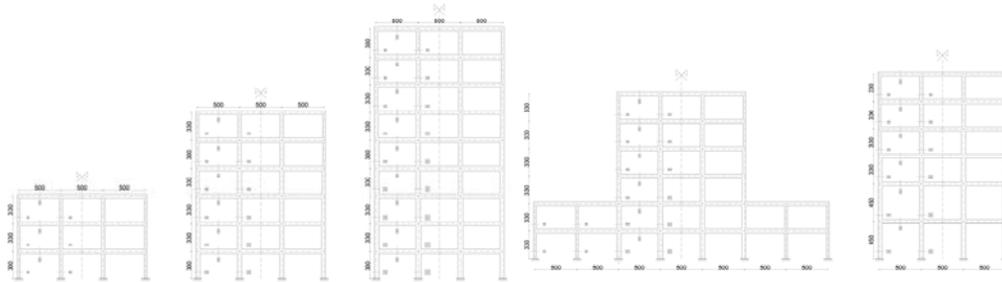
Figure 1. The case studies (regular frames 3F, 6F, 9F and irregular frames 6FIM and 6FIR).
