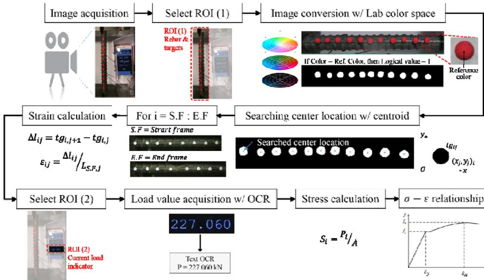
Figure 1. Algorithm for the image processing using colored target.
