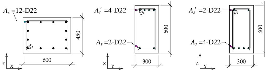
Figure 2. Details of (a) a-a' section; (b) b-b' section; and (c) c-c' section.
