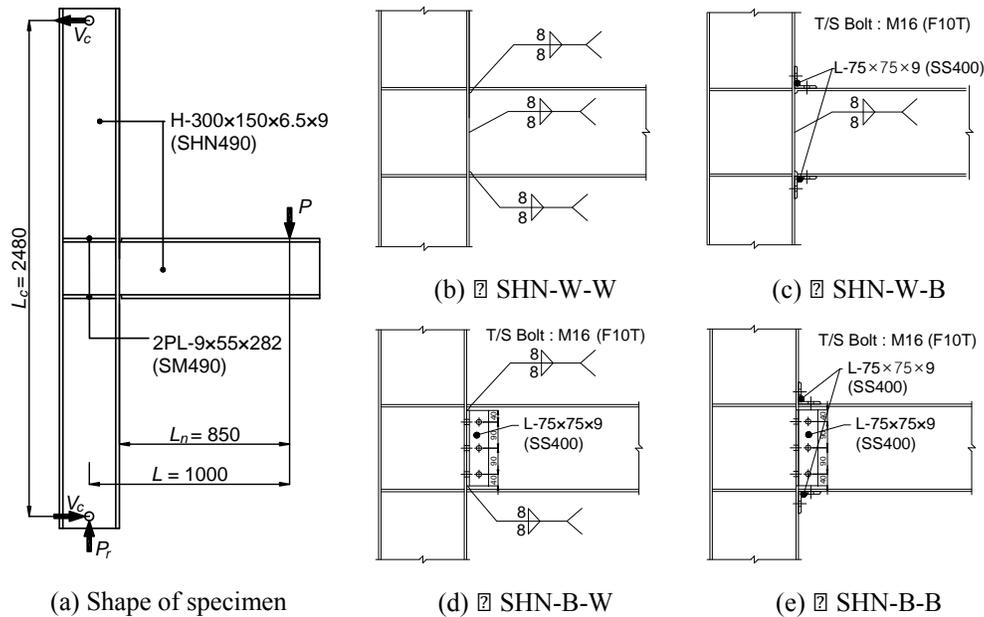
Figure 1. Shape of specimen and connection details.
