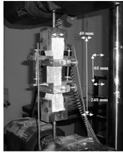
Figure 1. Direct tensile stress test setup with a displacement rate of 0.4 mm/min.
