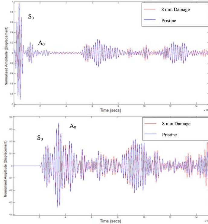
Figure 6. Comparison of damaged (8 mm delamination) and pristine specimen using the pulse-echo method (above) and the pitch-catch method (bottom) at an excitation frequency of 60 kHz.
