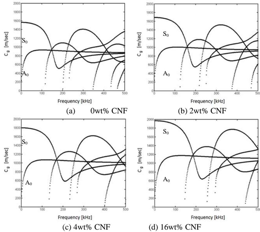
Figure 1. Dispersion curves of single-layer 4-mm-thick media.
