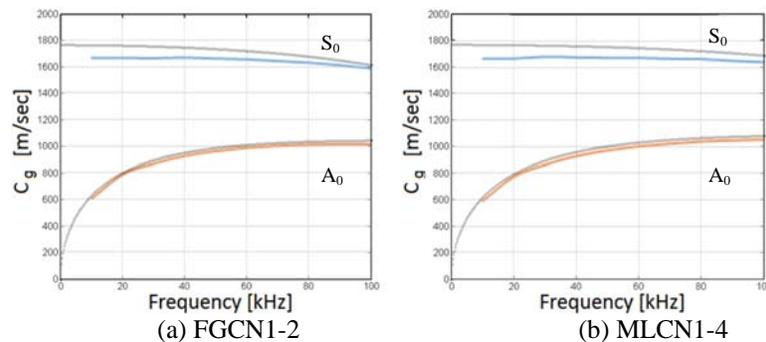
Figure 5. Dispersion curves of multilayered phenolic resin plates.
