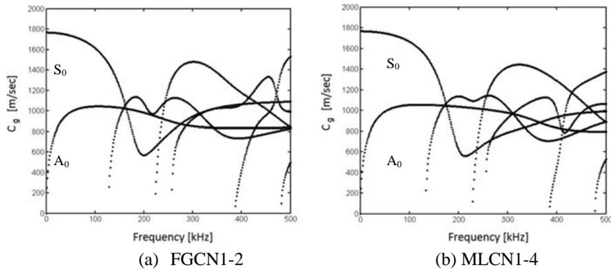
Figure 3. Dispersion curves of multilayered phenolic resin plates.
