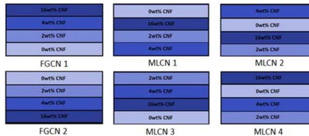
Figure 2. Graphical representation of multilayered phenolic resin media.
