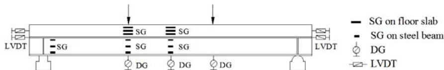
Figure 2. Location of strain gauges (SG), dial gauges (DG) and linear voltage displacement transducers (LVDT).
