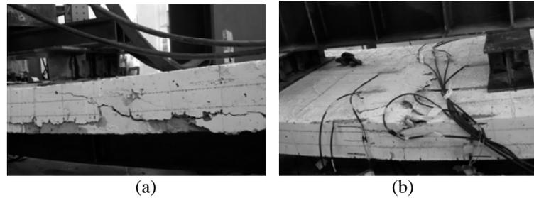
Figure 3. Typical failure modes: (a) diagonal shear crushing for SCB-1 with composite floor slab and (b) crushing of concrete for SCB-12 with cast-in-situ floor slab.
