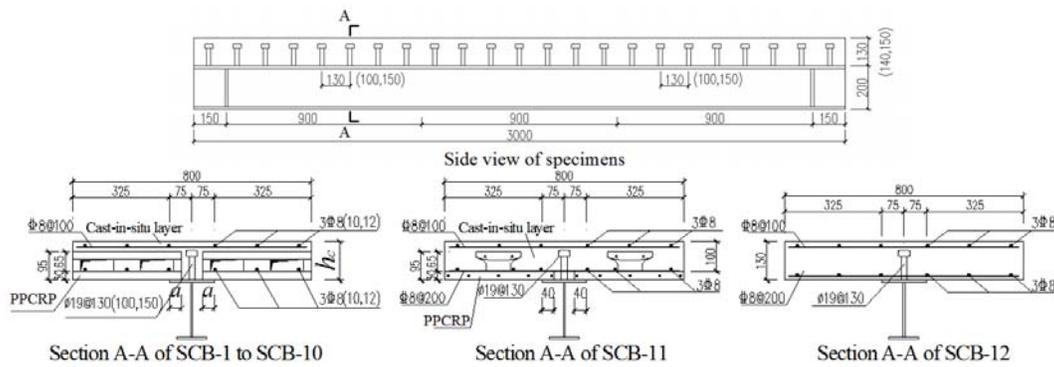
Figure 1. Sectional and reinforcement layout of specimens.
