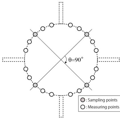
Figure 5. A measuring unit with 4 sampling points.
