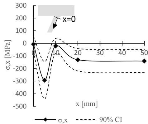
Figure 6. Transversal residual stress in the stiffener.
