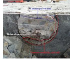
Figure 8. Shear connection failure in SCSGB 4.
