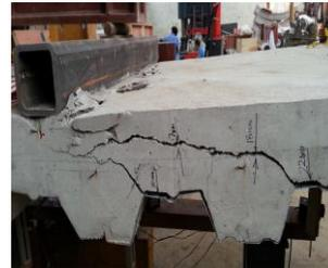
Figure 6. Failure mode of SCSFB 3.
