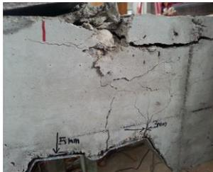
Figure 5. Failure mode of SCSFB 1.
