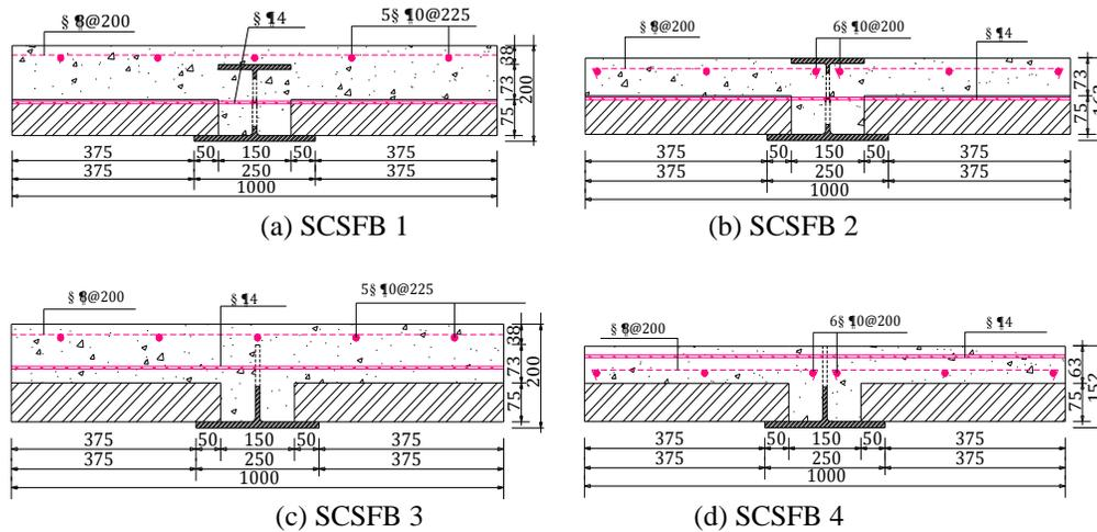
Figure 3. Geometrical characteristics of composite cross-sections.
