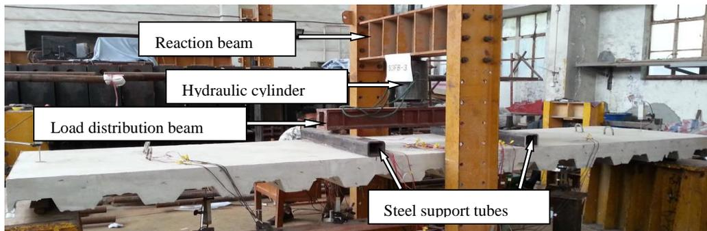
Figure 4. A shallow cellular beam specimen on the test frame.
