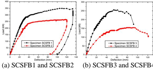
Figure 7. Load-deflection curves of the specimens.
