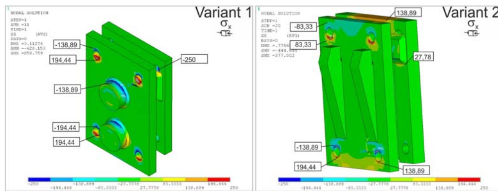
Figure 1. Results of numerical (FEM) analysis of steel connecting elements.
