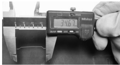
Figure 1. Hooked-end steel fibers used in fibrous mixes.
