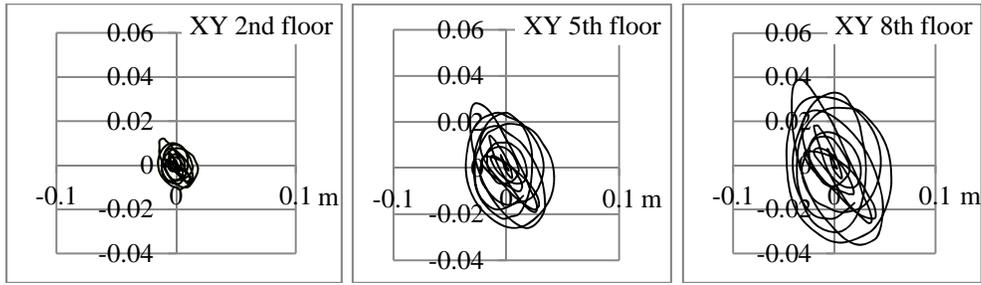
Figure 7. 2, 5, 8<sup>th</sup> floors XY displacement curves during El-Centro (N-S horizontal, E-W).
