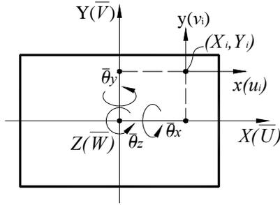
Figure 1. Slab center of mass and elements position.
