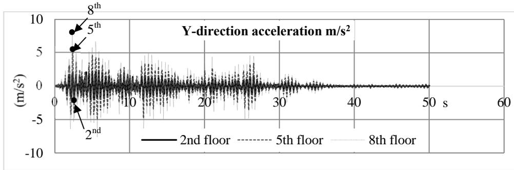
Figure 8. 2, 5, 8<sup>th</sup> floors acceleration responses during El-Centro (E-W component).
