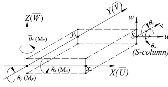
Figure 2. Freedom of element and slab.
