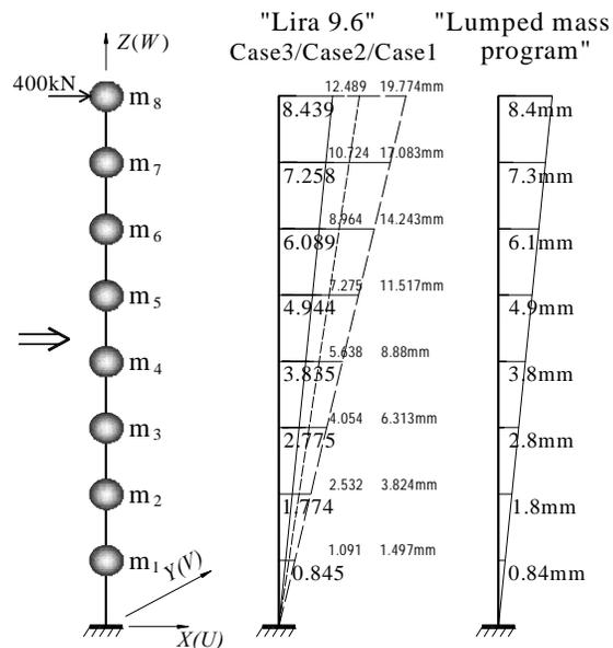
Figure 5. Comparison of displacement under static load.
