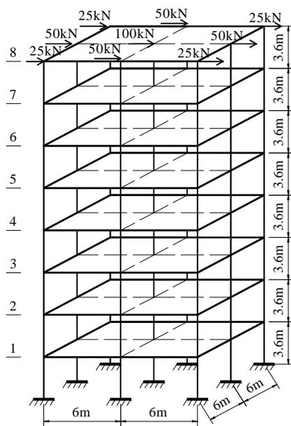
Figure 4. Analytical model of 8<sup>th</sup> floors building.
