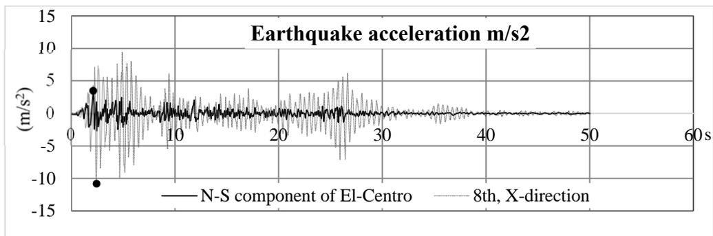
Figure 6. 8<sup>th</sup> floor and ground acceleration responses during earthquake (N-S component).
