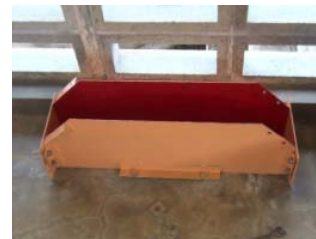
(c) Bottom of molding box.
