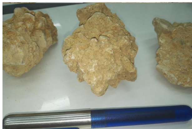
Figure 5. The Sarooj mortar elements and aggregations in comparison with the size of a pen.
