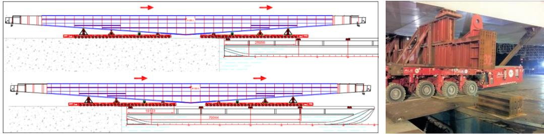
Figure 3. Sketch of two stages of the load-out (left) and picture of the SPMTs reaching the barge (right).
