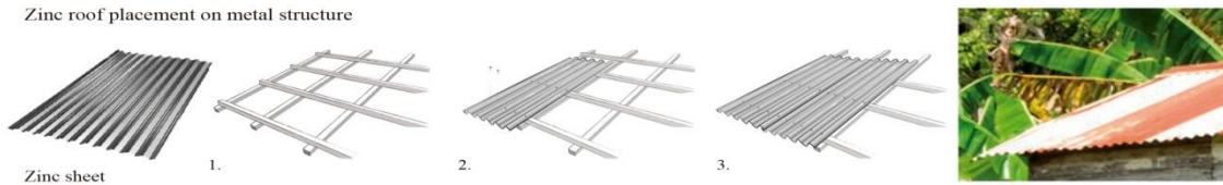
Figure 3. Zinc roof construction process.
