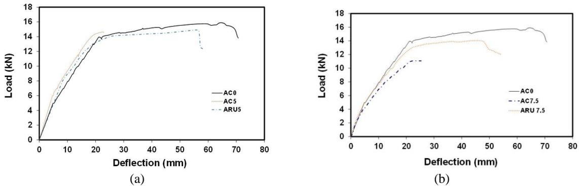
Figure 4. Effect of CFRP U-wrap strips on beams without stirrups (a) Beams with 5% corrosion; (b) Beams with 7.5% corrosion.
