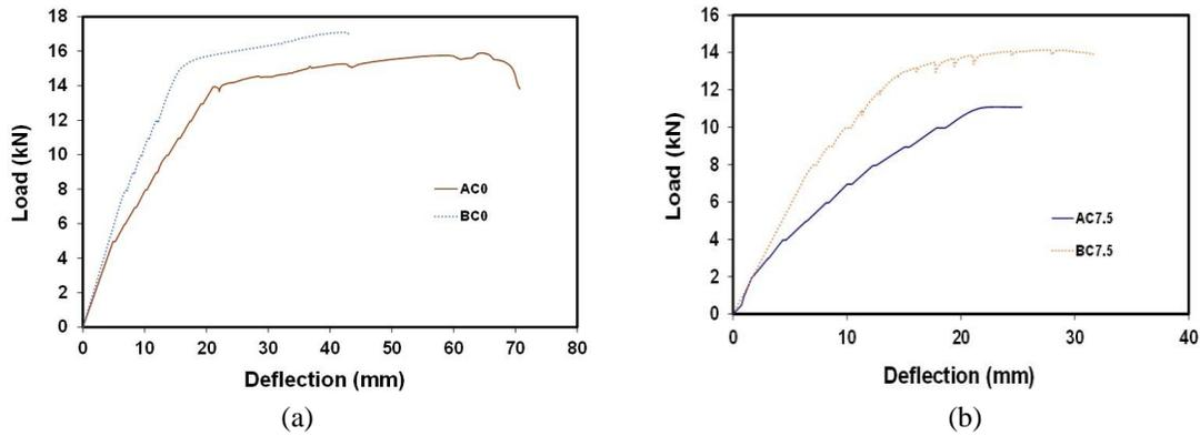
Figure 3. Effect of stirrups on beams (a) control; (b) corroded.
