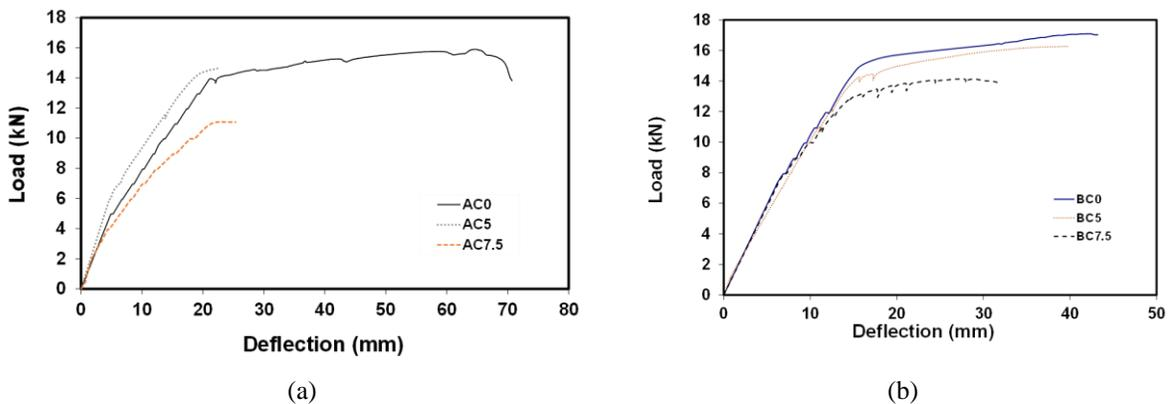
Figure 2. Effect of corrosion (a) Beams without stirrups; (b) Beams with stirrups.
