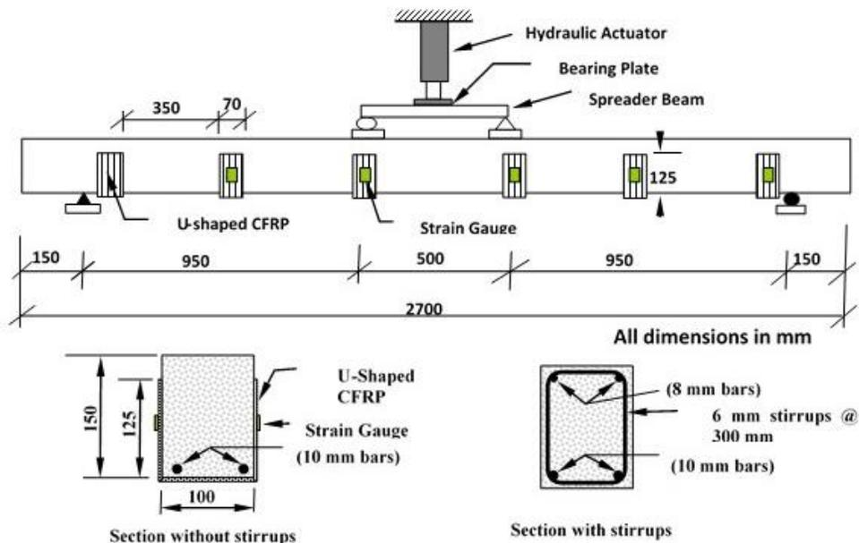
Figure 1. Test setup for beams and cross section details.
