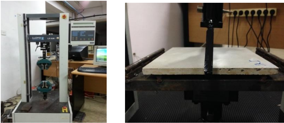
Figure 2. Experimental setup: (a) test machine (b) small concrete plate.
