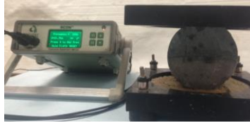
Figure 2. Electrical resistivity testing of ECC cylindrical specimens.
