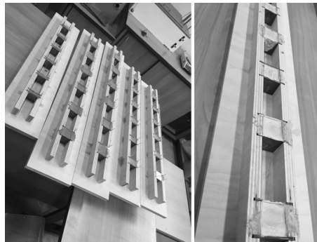
Figure 1. Molds for pull – clamping test samples.
