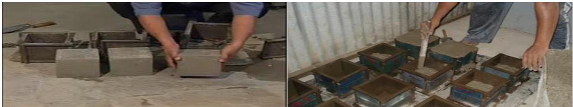
Figure 1. Preparation of samples for compressive strength testing.
