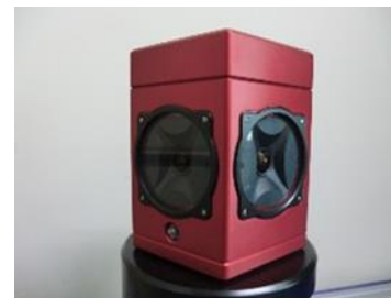
Figure 2. All-around view camera.
