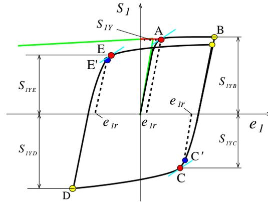
Figure 2. Deviatoric stress-deviatoric strain curve in the first cycle.
