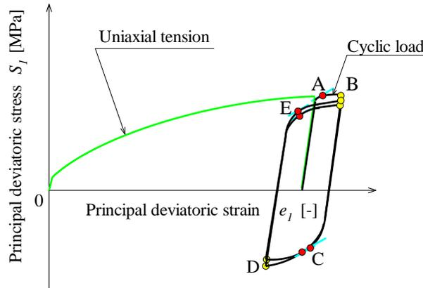
Figure 1. Cyclic loading tests for tension and compression after pre-deformation of uniaxial tension.
