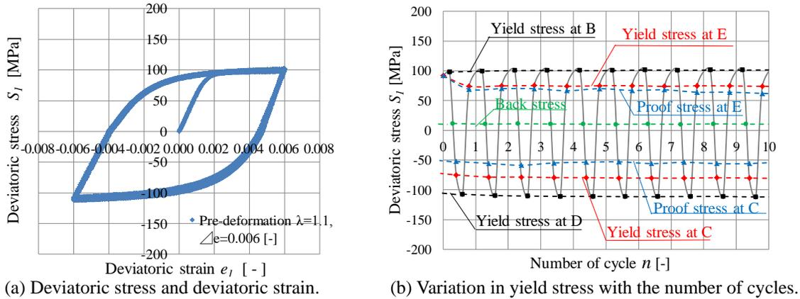
Figure 5. Variation of yield stress in cyclic loading for tension and compression ( $\lambda=1.1$ ,  $\Delta e_I = 0.006$ ).
