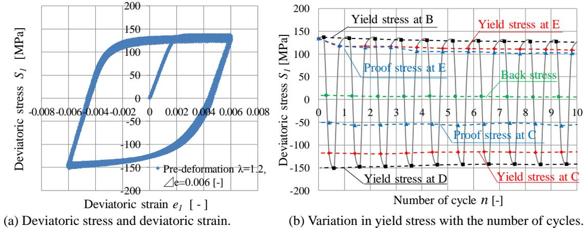
Figure 4. Variation of yield stress in cyclic loading for tension and compression ( $\lambda=1.2$ ,  $\Delta e_I = 0.006$ ).
