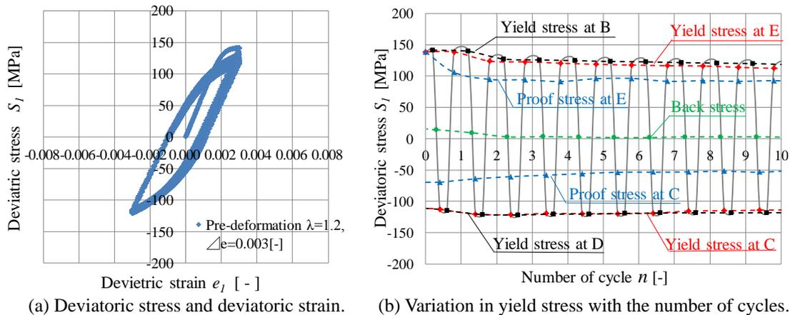
Figure 6. Variation of yield stress in cyclic loading for tension and compression ( $\lambda=1.2$ ,  $\Delta e_I = 0.003$ ).
