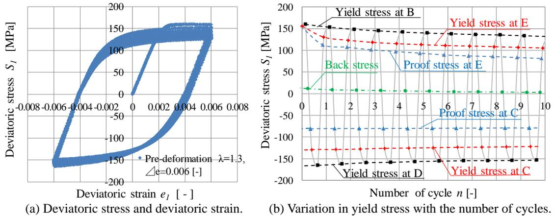
Figure 3. Variation of yield stress in cyclic loading for tension and compression ( $\lambda=1.3$ ,  $\Delta e_I = 0.006$ ).
