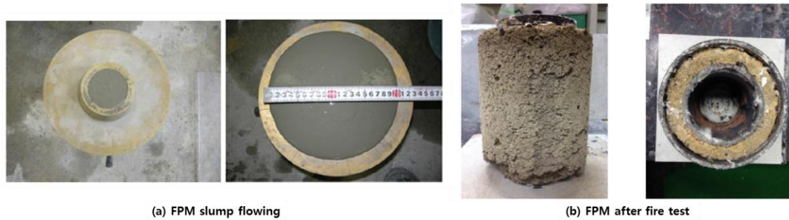
Figure 1. Fire protection mortar.
