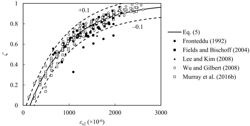
Figure 2. Evolution of scalar damage parameter  $\zeta$  with increasing load.
