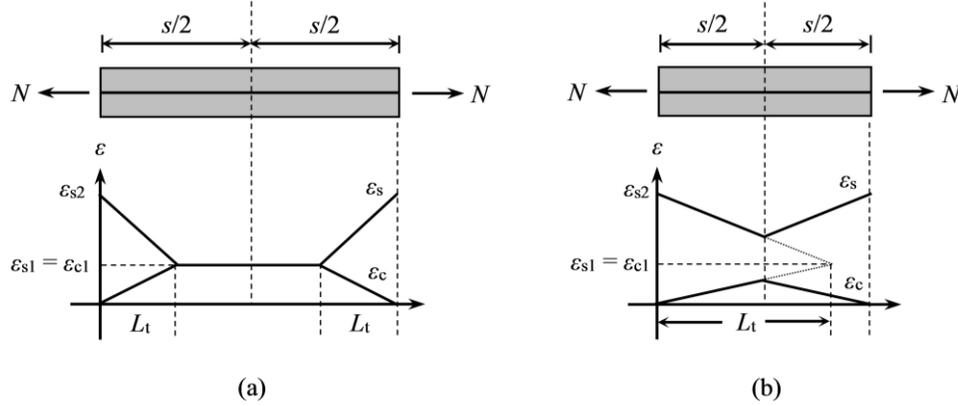
Figure 1. Reinforcement and concrete strain in (a) a long segment and (b) a short segment.
