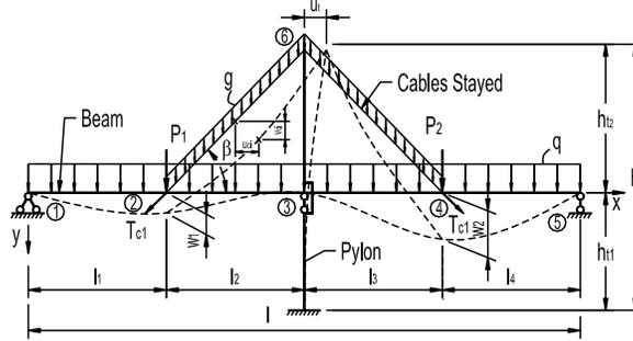
Figure 3. Plane cable-stayed structure.
