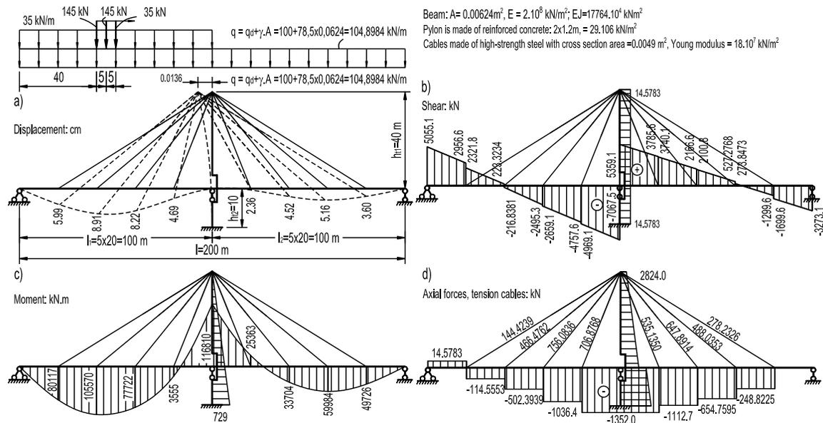
Figure 4. Cable-stayed structure in numerical example.
