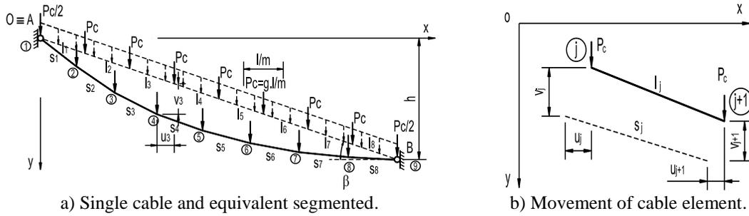
Figure 1. Inclined single cable subjected to self-weight.
