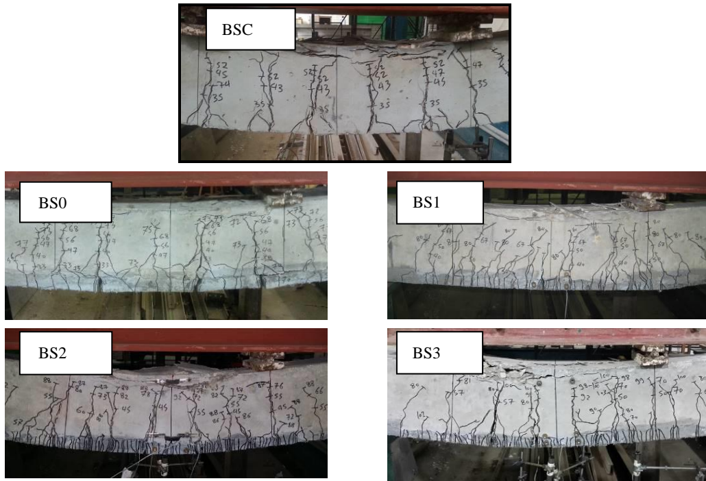
Figure 2. Cracks pattern and failure mode of tested beams.
