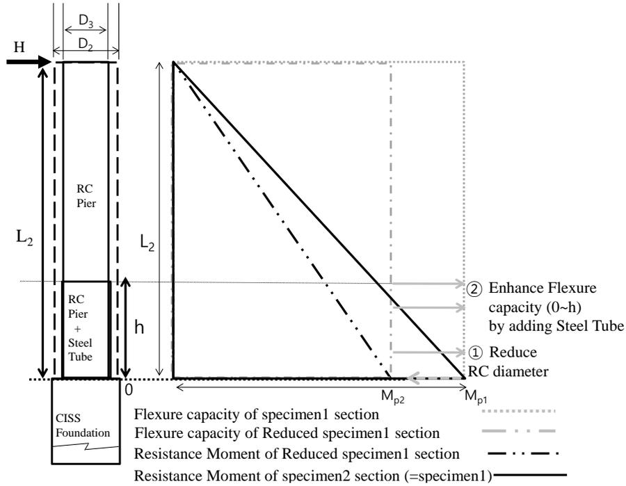
Figure 3. Bending moment diagram of specimens.
