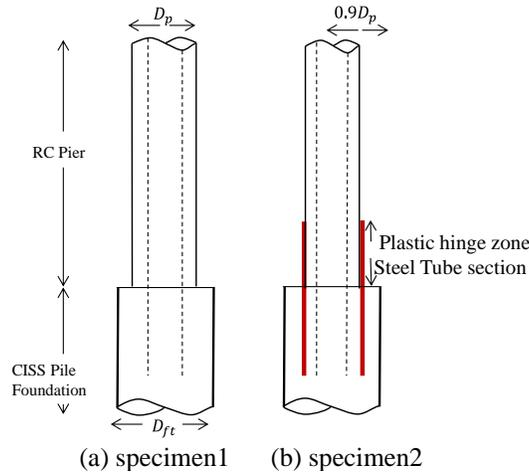
Figure 1. CISS foundation - RC pier connection and steel tube.
