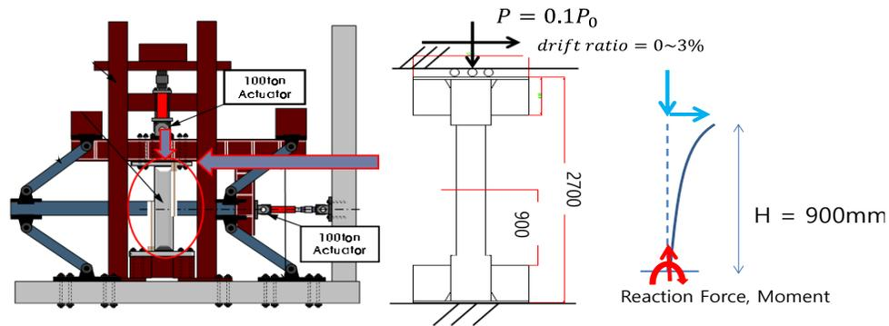
Figure 4. Diagram of axial-bending test frame and loading summary.
