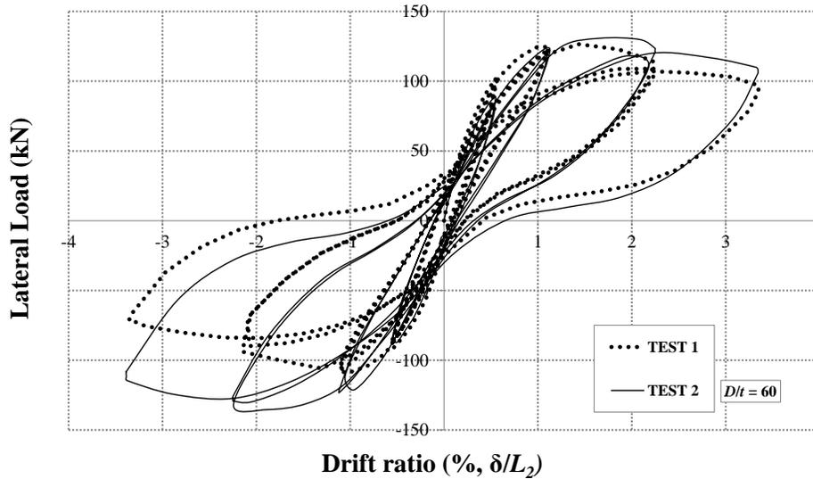
Figure 6. Later reaction force-drift curve of specimen 1 and 2.
