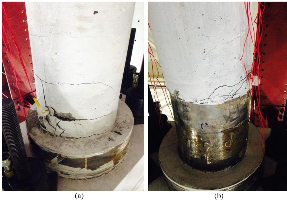
Figure 5. (a) Deformed specimen 1 and (b) deformed specimen 2 (steel tube).
