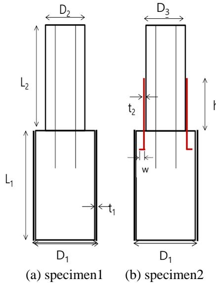
Figure 2. Geometry of specimen 1 and 2.
