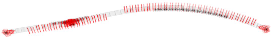
Figure 8. Deformation and cracks on Sarch under one point loading.
