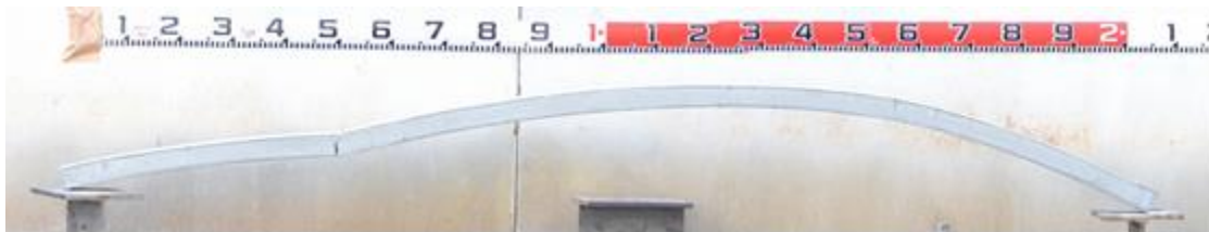
Figure 5. Deformation and cracks on Sarch under one point loading.
