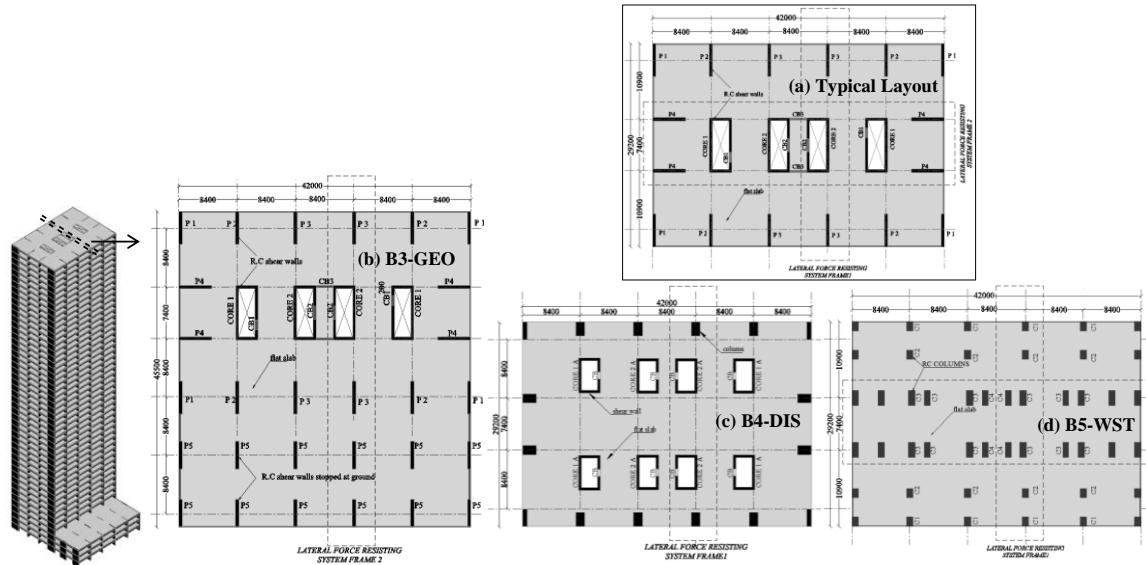
Figure 1. Selected reference structures: (a) typical layout; (b) B3-GEO configuration and layout, (c) B4-DIS layout at the irregularity level, and (d) B5-WST layout at the irregularity level.
