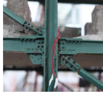
Figure 3. Photograph of BRB connection.
